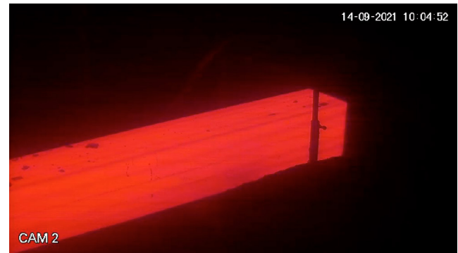
Fig. 2. Image example of billet from the descaler.
